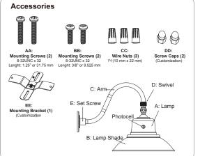
Connect Arm (C) and Lamp (A) through Swivel (D) and rotate Swivel to fasten two parts. Be careful not to misplace any of the hardware needed for installing the fixture
