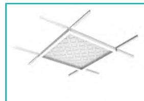
2 SCXT-L2FT INSTALLED ON T-BAR CEILING
